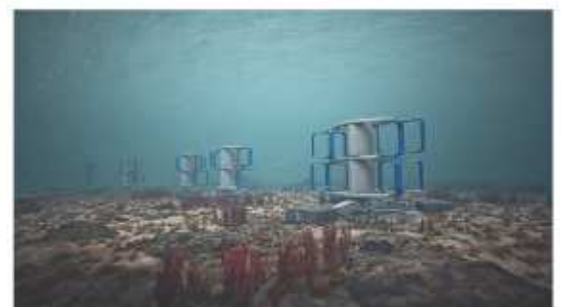
Artist's rendering of the pilot farm FloWatt project based on 2.5 MW capacity turbines deployment in the Alderney Race (English channel, France).
